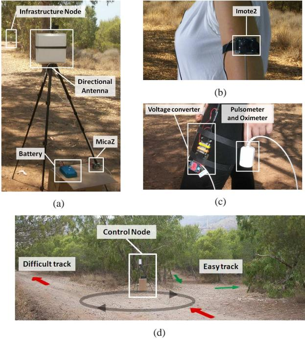
Fig. 3: Deployed hardware. 3(a) Infrastructure node. 3(b) Upper User Equipment. 3(c) Lower User Equipment. 3(d) Crossroad.
