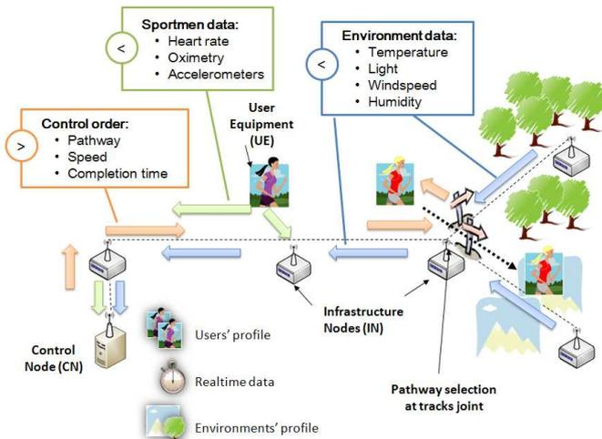
Fig. 1: Data flow of the sensed data, and, the commands flow from the CN.
