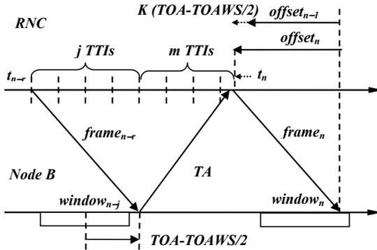
Fig. 2. Time diagram of the offset adjustment algorithm
