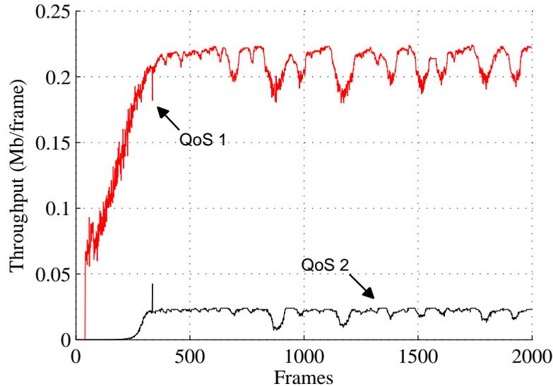
**Figure 4.** Trace of the throughput per MAC frame for each QoS class. QoS1 and QoS2 are granted 90% and 10% of the resources respectively.
