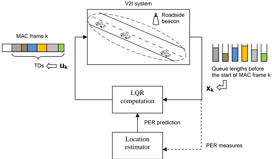
**Figure 2.** Diagram of the feedback structure of a LQR-based V2I scheduler and the variables involved.
