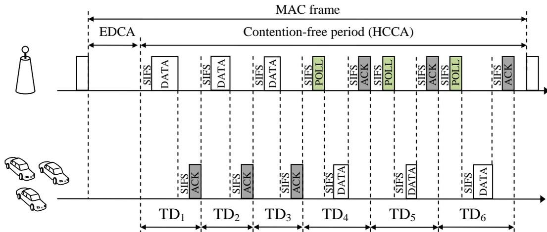
**Figure 1.** Simplified temporal diagram of a MAC frame allocating 3 downlink and 3 uplink TXOPs.
