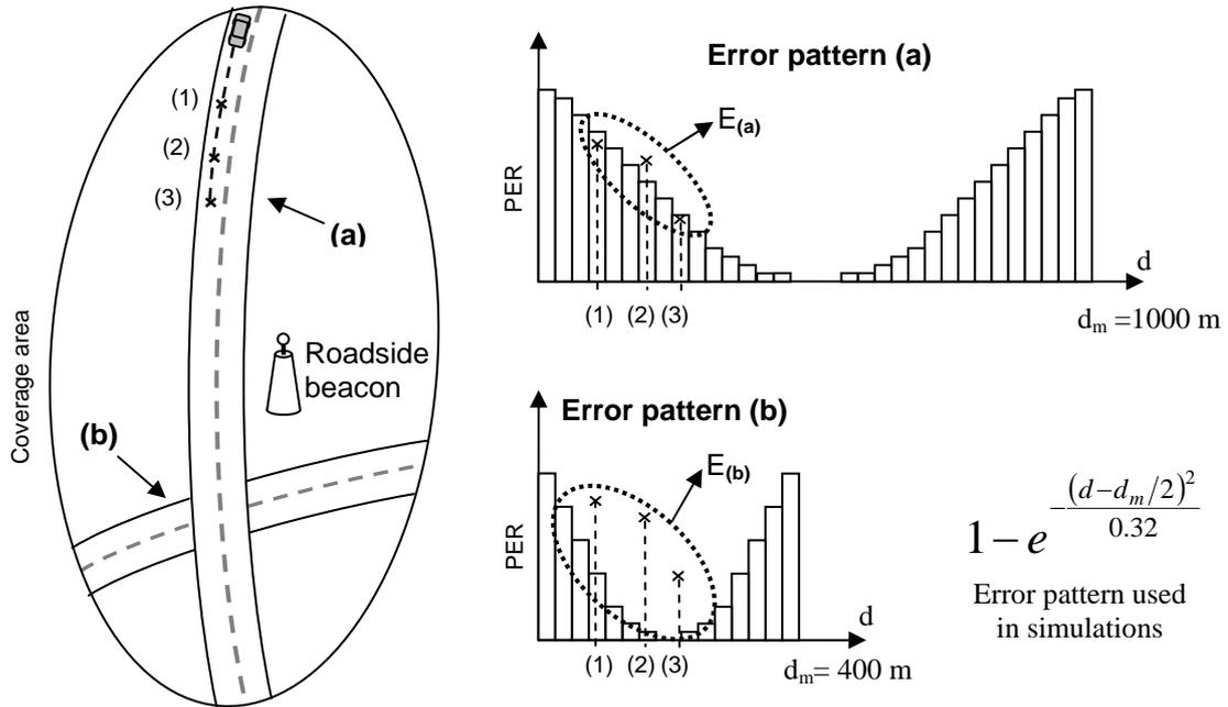
**Figure 3.** Example scenario with a roadside beacon covering two road segments of different lengths. The system obtains PER measurements for a vehicle when it transmits or receives a burst of MSDUs. The system compares these measures with the stored error patterns of each route. In this case, the system detects very fast that the vehicle moves along route (a).
