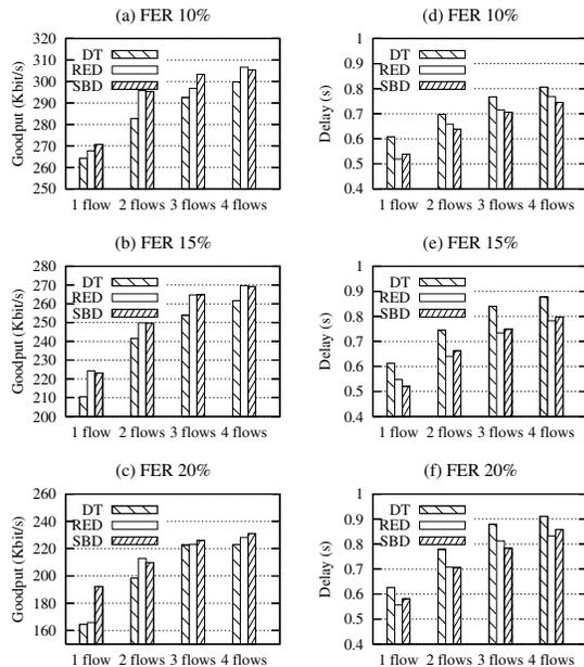
Figure 8. TCP Reno performance vs. FER. 40 SDUs buffer.
