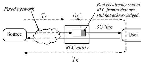
**Figure 2. Diagram of the end-to-end connection**
